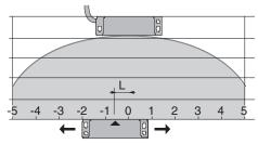
5 mm misalignment tolerance after setting
