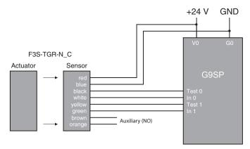
Series connection Application, up to 3 Sensors with G9SP (up to Safety PLd acc. EN ISO 13849-1)
